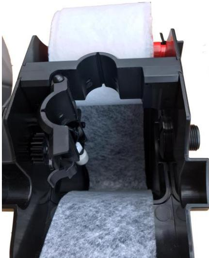
The new roll is now inserted. The fleece is directed from the new roll downwards. Hold the end of the fleece tight while remounting the inlet pipe. This presses the fleece to the bottom towards the grid. If the inlet pipes are in the right position, you can close the clip. Now you can tear the fresh end of the fleece and wind it round the receiving roll. You can use a piece of tape to fix it there. The receiving roll is now pressed into its place so that the gear
