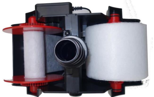
The fleece is transported from the releasing roll to the accepting roll. The rolls are driven by gear wheels by gear wheels. If the accepting roll is full – or the releasing roll empty, it can be taken out of the filter easily. Both parts can be separated and the fleece can be discarded.
