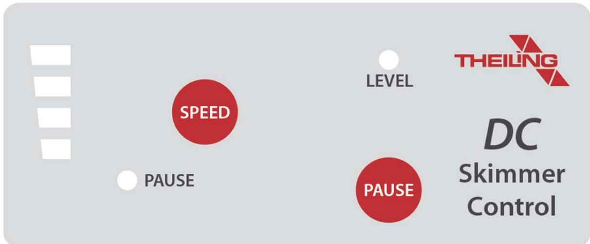
The pump controller DC Skimmer Control enables you to control the rotation speed of the venturi pump of the ECONE 3000 DC protein skimmer and adjust in this way the foam production.
